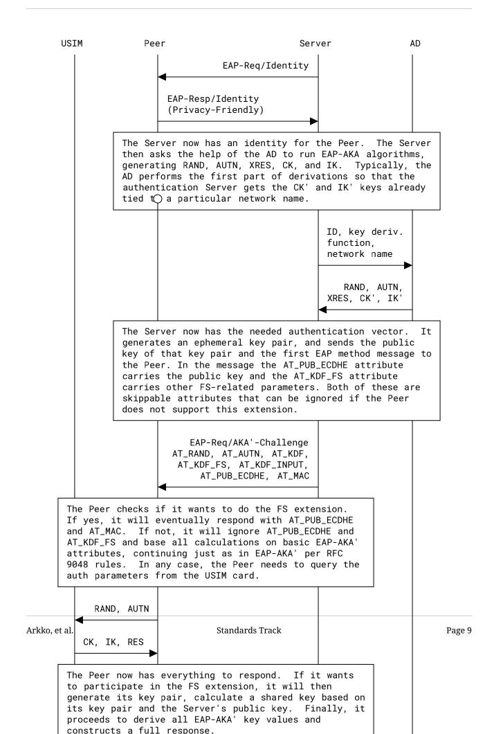
Figure 2: EAP-AKA' FS Authentication Process
